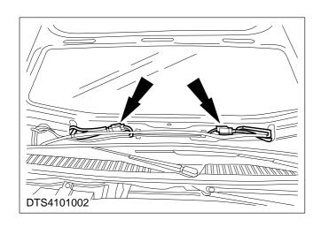
4. Disconnect the two heated screenwash jet multiplugs.
