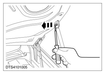
7. Support the hood and disconnect the two damper struts.
