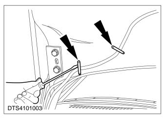
5. Unclip the screenwash tube and harness from the hood.
