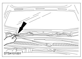
3. Disconnect the screenwash tube at the T-joint and unclip from the hood.
