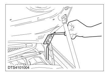
6. Using a suitable marker pen, mark the position of the hood hinge brackets.
