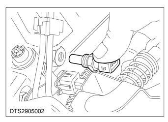
4. Unscrew and remove the ECT sensor.
