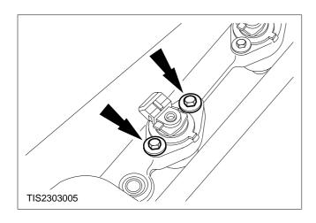
8. Remove the two fuel injector retaining bolts.
