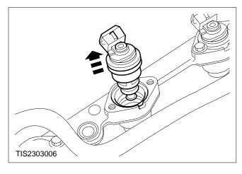
9. Remove the fuel injector/injectors.
