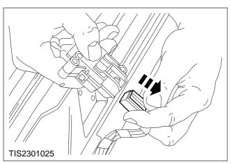
CAUTION: Do not pull on the wiring; pull on the multiplug body.
