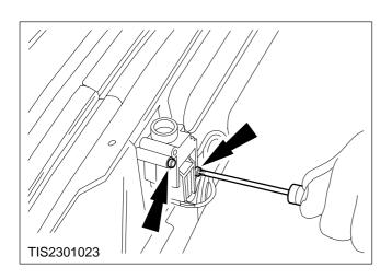
4. Unscrew the fuel shut off switch retaining screws.
