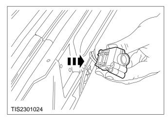
5. Remove the fuel shut off switch from the rear panel.
