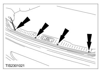
2. Unscrew the trim panel retaining screws.
