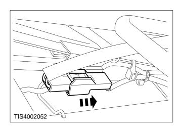
4. Remove the seat belt stalk (two Torx bolts).
